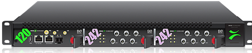
Figure - The Enhanced Chassis populated with one VB120 controller blade and two VB242 ASI input modules giving a total of 5 ASI inputs concurrently monitored. Alternatively 12 inputs monitored in a round-robin fashion plus one VB120 ASI input concurrently monitored locally on the VB120 module (HD-BNC input).
