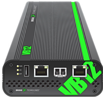
Picture: the VB12 unit with both SFP based Optical GigE or Electrical auto-switching 10/100/1000-T Ethernet interfaces, separate 10/100-T management interface, RS232 based USB connector for setup and status LEDs.
